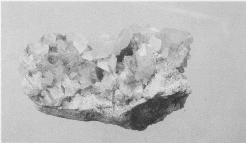
Figure 5: A specimen of well crystallised dolomite on quartz with some original clay matrix still adhering. The specimen is 10 cm long
